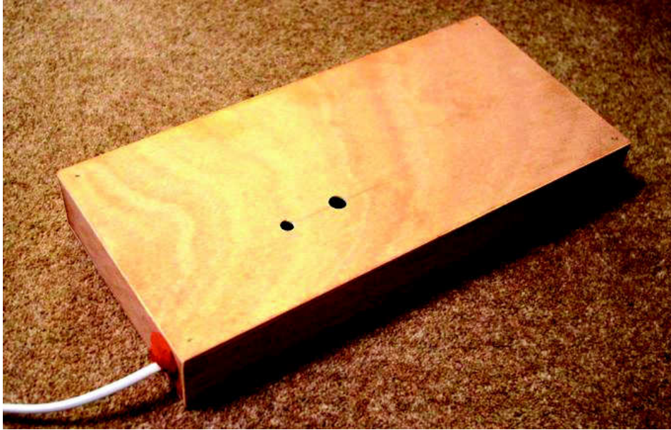
Figure 28: Plywood Box A with 9 and 11 mm holes, and cable for internal electret microphone.
