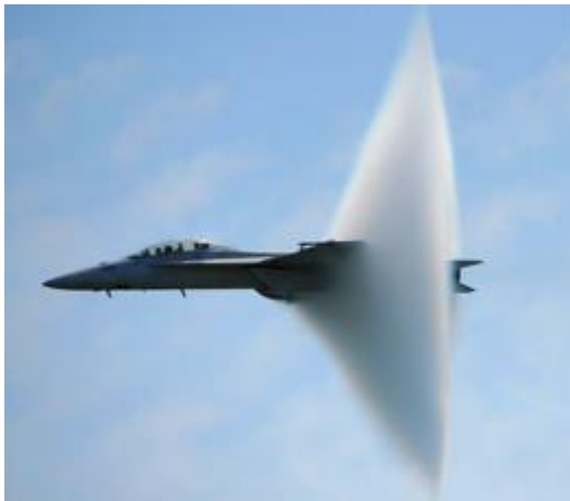
Figure 19 showing a transonic transient shockwave formation at M 1.08 at maximum area point
